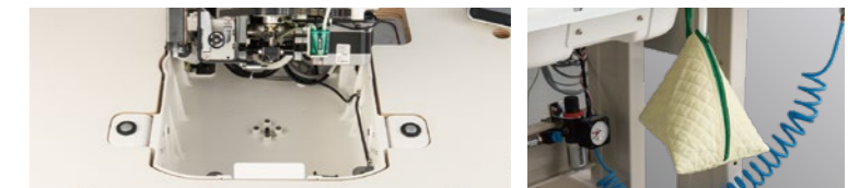
The wiring inside and outside the machine head is neatly tucked away under the machine head for easy cleaning.
